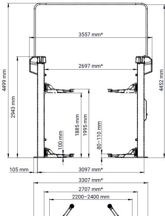
\*Dimensions refer to recommended drive-through width of 2400 mm
