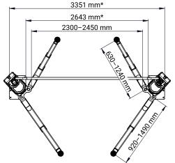
\*Dimensions refer to recommended drive-through width of 2400 mm
