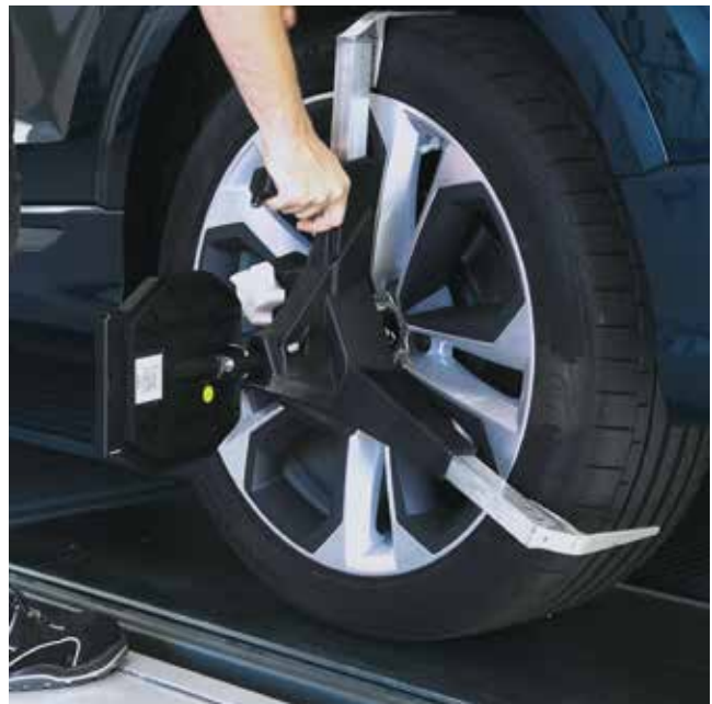
Q.Grip: safe, firm hold on the wheel
