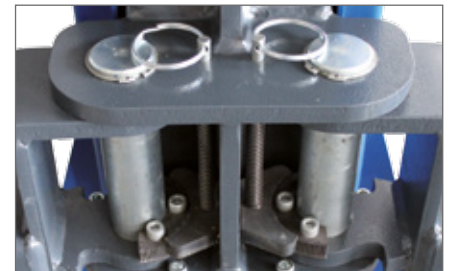
Automatic support-arm restraint with fine adjustment and manual release
