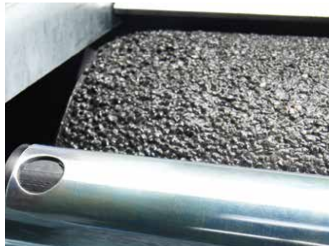
Wear-resistant rollers coated with plastic/corundum
