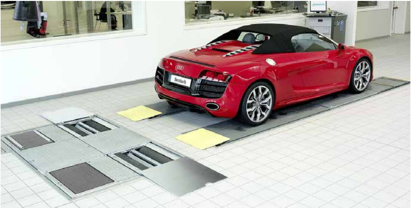
Theta suspension tester as alternative for EUSAMA measurement
