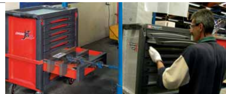
The drawers are tested over 50,000 opening / closing cycles, i.e. 10 years of use.
