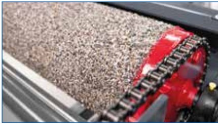
Roller surface plastic/granulate coated
