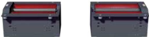
Digital roller brake tester C_MBT S 15.0 R100 MU with two-part roller set, up to 15.0 t axle load and a roller length of 1000 mm, motor positioned under the roller set.
