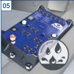
05 Encased, splash-resistant and almost completely waterproof interface module.
